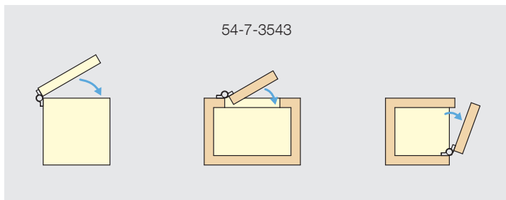
Damper working direction when opening the hinge
